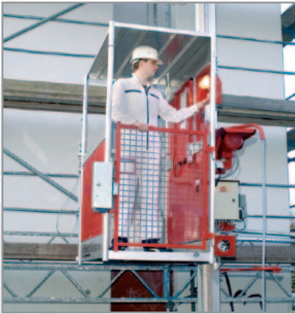
Swivel door with electro mechanical interlocking (entry side) and electrical controlled loading ramp (exit side)
